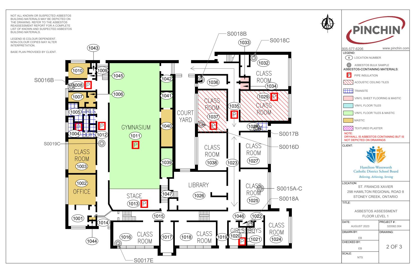
NOT ALL KNOWN OR SUSPECTED ASBESTOS BUILDING MATERIALS MAY BE DEPICTED ON THE DRAWING. REFER TO THE ASBESTOS REASSESSMENT REPORT FOR A COMPLETE LIST OF KNOWN AND SUSPECTED ASBESTOS BUILDING MATERIALS.
